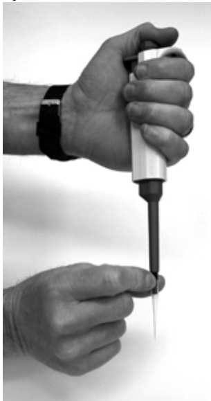
Hold the pipette with two hands
